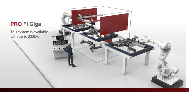
The PRO FI Giga is a unique system that can be highly customized to the needs of the customers. It offers different loading concepts, from vertical to horizontal, and a high degree of automation for direct integration into manufacturing lines.
